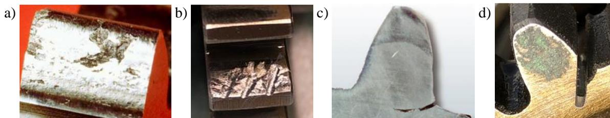
Fig. 3. Actual (a, c) and simulated (b, d) tooth damages
