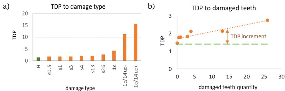
Fig. 4. Diagnostic parameter dependence on damaging (a), damaged teeth quantity (b)
