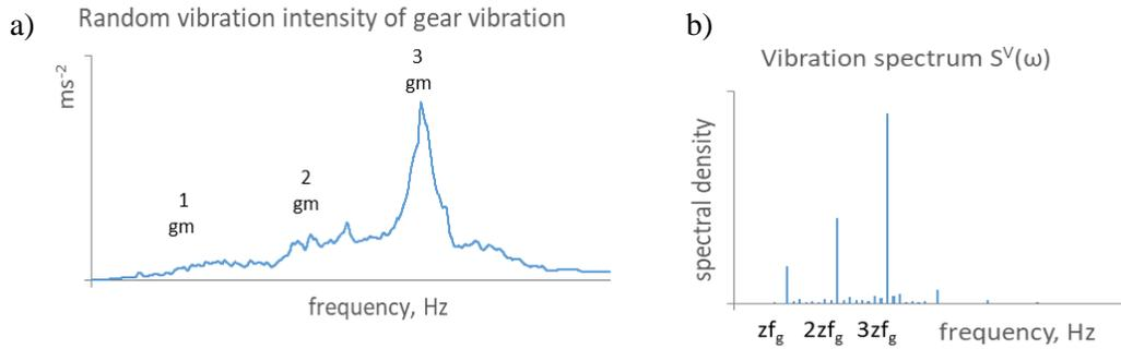
Fig. 2. **Vibration of the gear: random component (a), vibration spectrum (b)**
