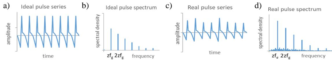
Fig. 1. **Ideal (a, b) and real (c, d) gear mesh model:**
